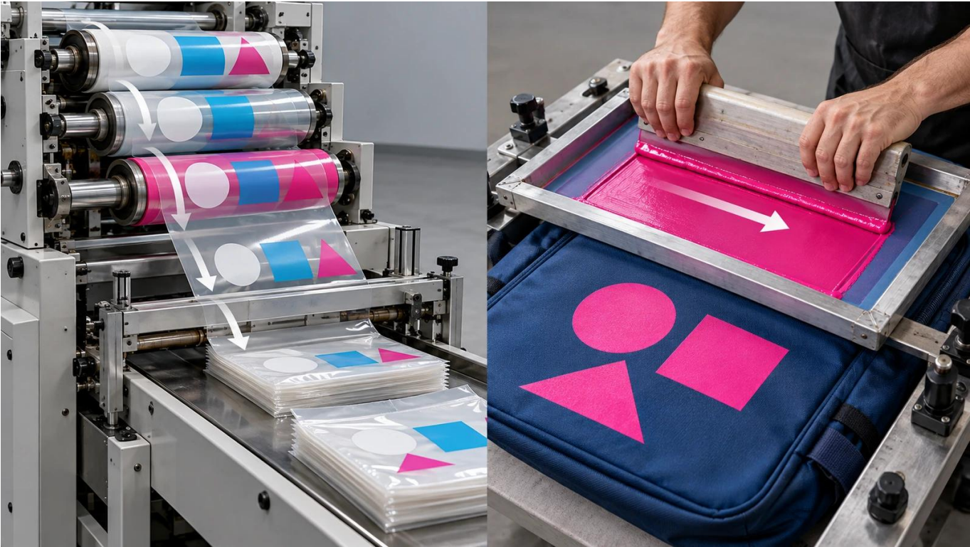
Figure 4: The process of creating a custom-printed bag. The left image shows a machine printing a design onto a roll of material. The right image shows a person using a squeegee to apply ink to a bag.
